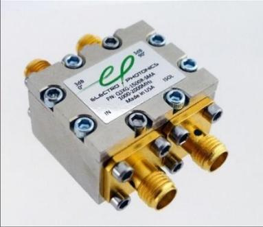
A 90 degree hybrid coupler is a four-port device used to equally split an input signal into two signals with a 90 degree phase shift between them. The 90 degree hybrid coupler can also be used to combine two signals while maintaining high isolation between them.
