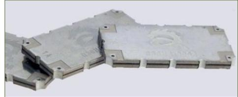
Most surface-mount hybrid couplers use a multilayered broadside coupling construction in comparison to a microstrip edge coupled structure. Typical construction of a hybrid coupler consists of two transmission lines in close proximity. RF energy travelling through one of the transmission lines couples to the other transmission line. There is a 90° phase difference between the output ports of a hybrid coupler.
