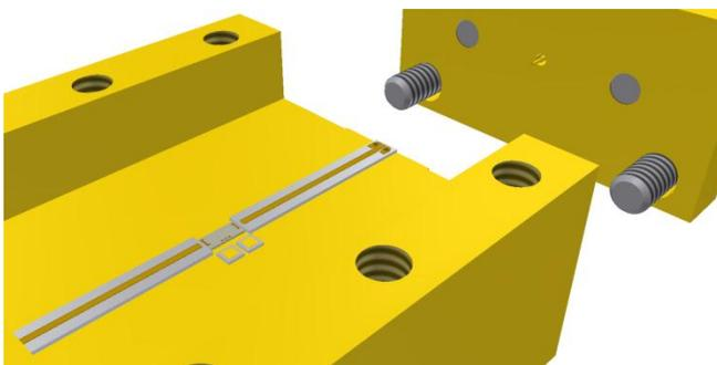
Fig 2: Launch assembly removed for probe access
